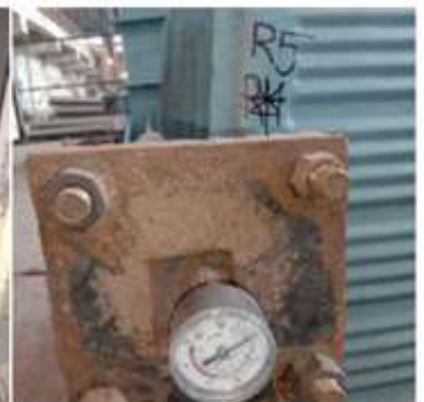
Pressure test for leaks in radiator
